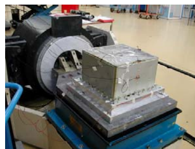
Vibration test of FMA structure
