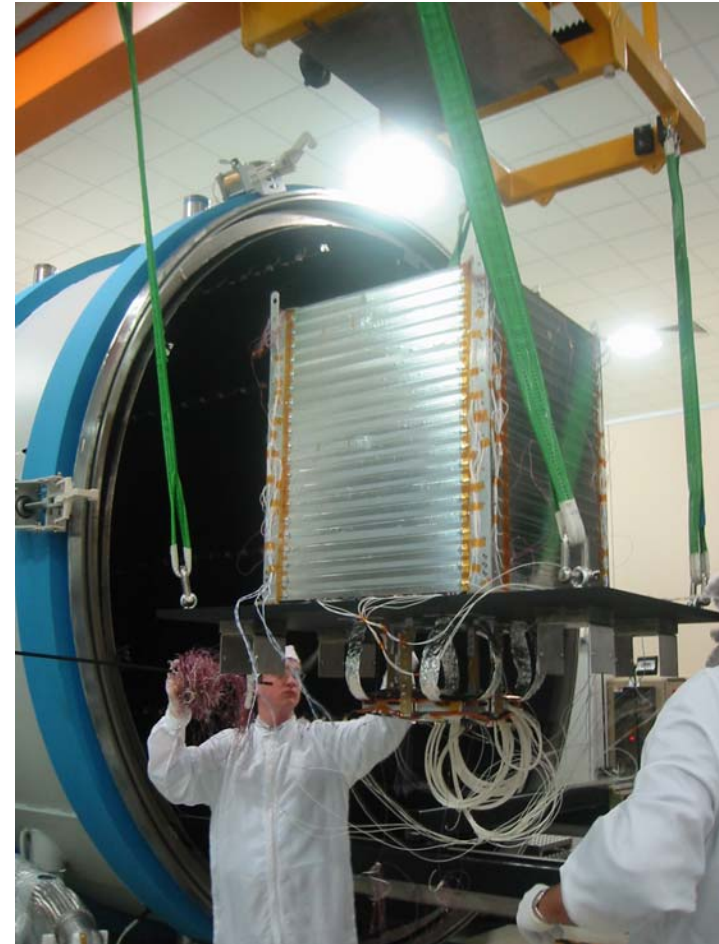
Engineering Model at Alenia for T/V test
