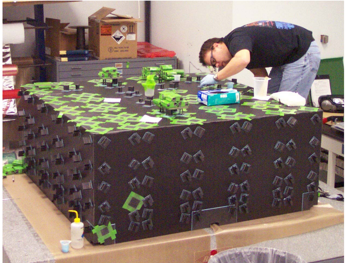
Flight composite shell, with tile mounting flexures being bonded.
