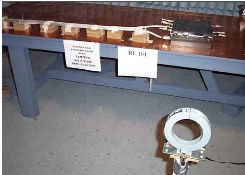
Radiated Emissions Test Setup
