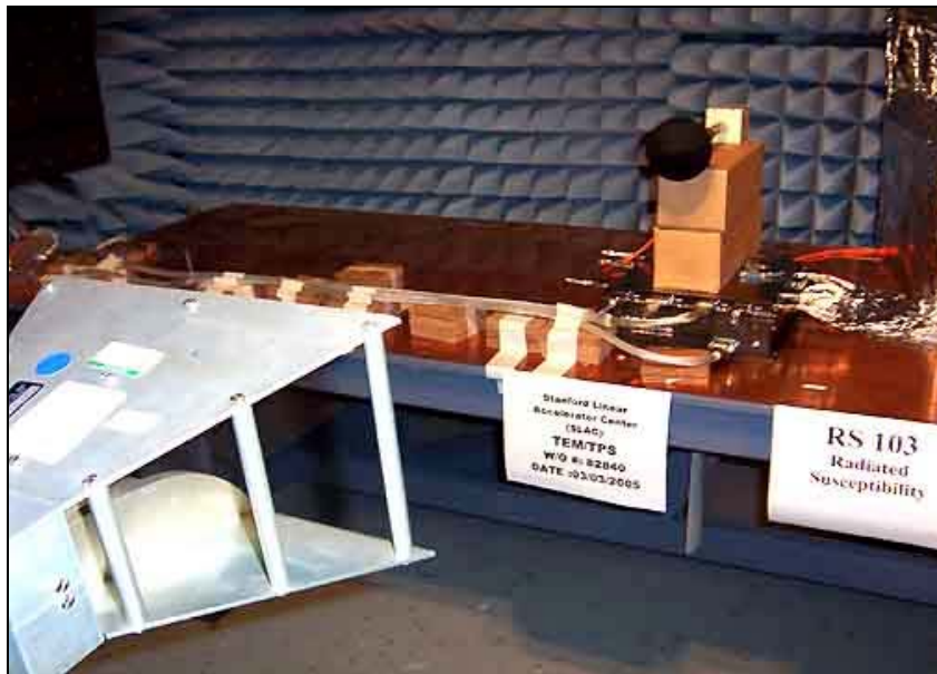
Horn Antenna, 1 - 18GHz Vertical Polarization Test Setup
