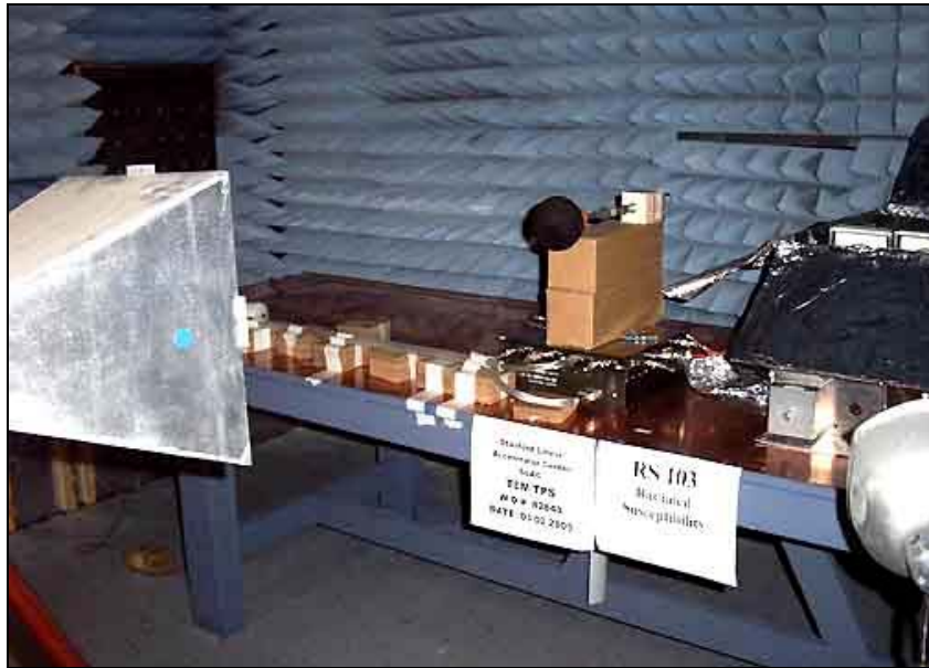
Horn Antenna, 1 - 2GHz Horizontal Polarization Test Setup
