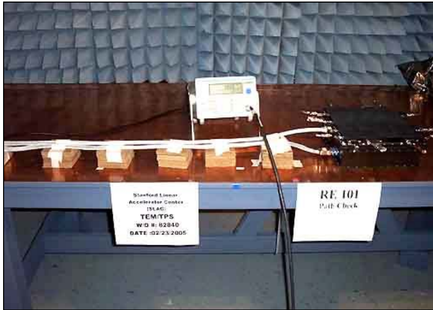
Radiated Emissions Path Check
