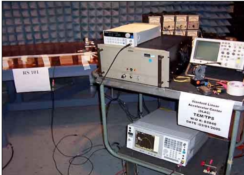
Radiated Susceptibility Test Equipment
