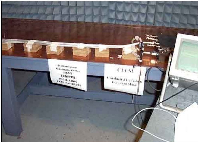
Conducted Emissions Common Mode Test Setup
