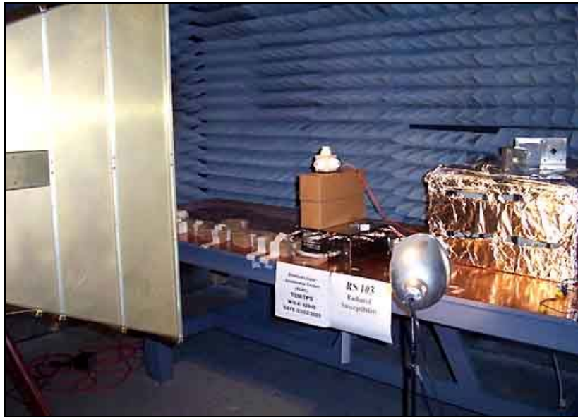
Horn Antenna, 200 - 1000MHz Horizontal Polarization Test Setup
