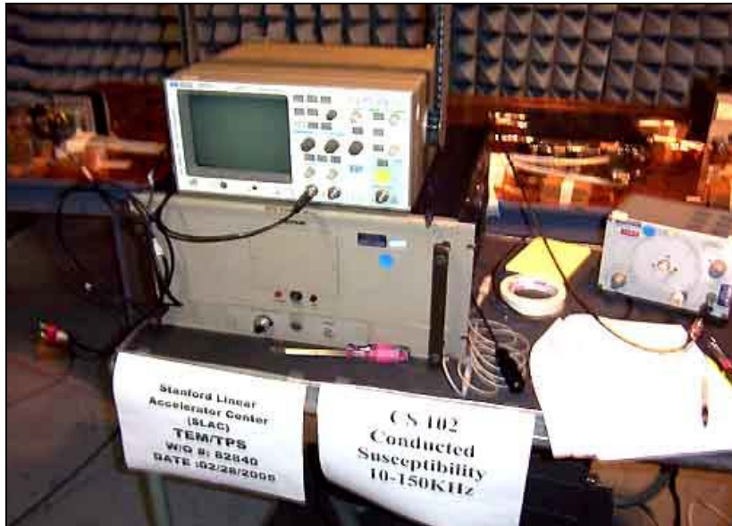
CS102 Test Equipment Closeup
