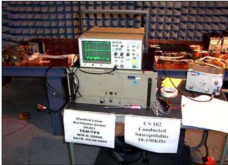
CS102 10 - 150kHz Test Setup
