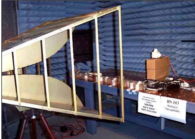
Horn Antenna, 200 - 1000MHz Vertical Polarization Test Setup
