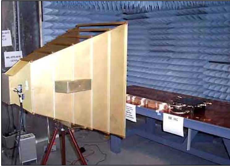
Horn Antenna, 200 - 1000MHz Horizontal Polarization Test Setup
