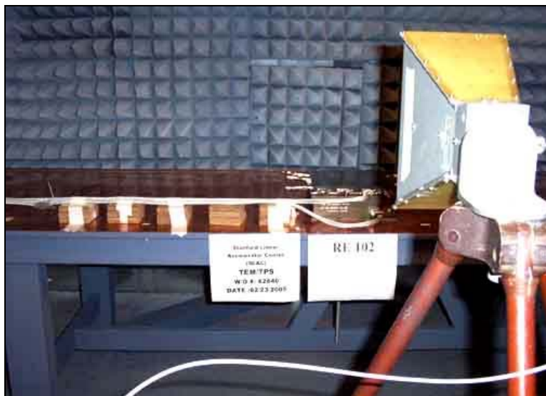
Horn Antenna, 1 - 18GHz Horizontal Polarization Test Setup
