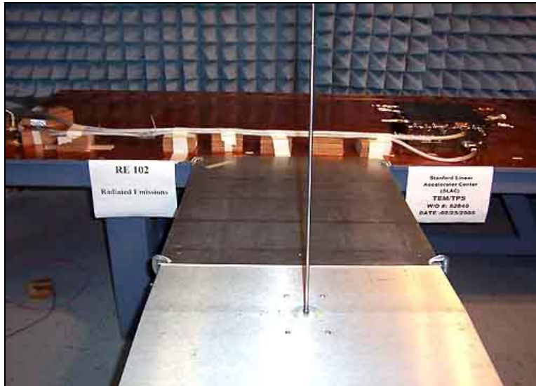
Rod Antenna, 10kHz - 30MHz Test Setup
