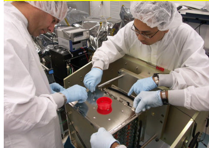
Installation of EMI Side Panels – lots of fasteners
