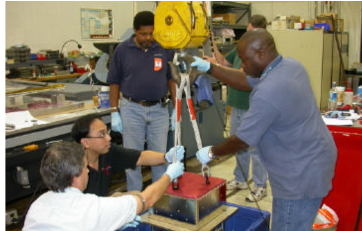
Remove FMA from shipping container for vibration testing
