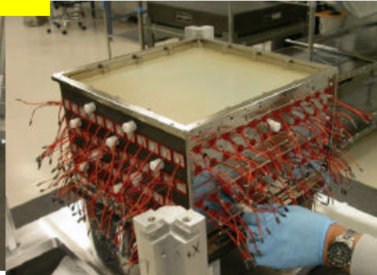
Closeout plates keep CDEs in place
