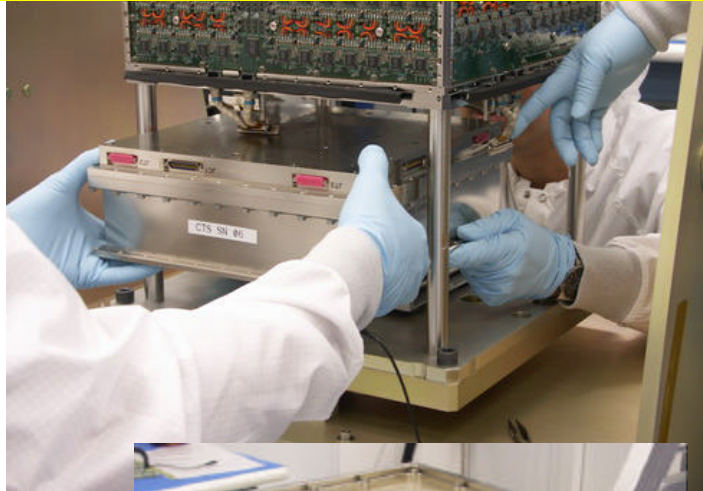
Installation of SLAC's EM2 TEM/TPS
