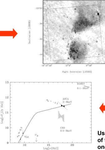
More detailed Chandra X-ray contors overlaid on VLA 21 cm radio map (nonthermal). Source 5 is the candidate, after elimination of others as unlikely gamma-ray sources from optical observations.
