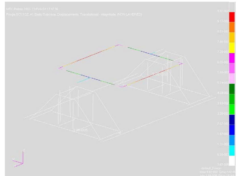
Displacements under 1gz
