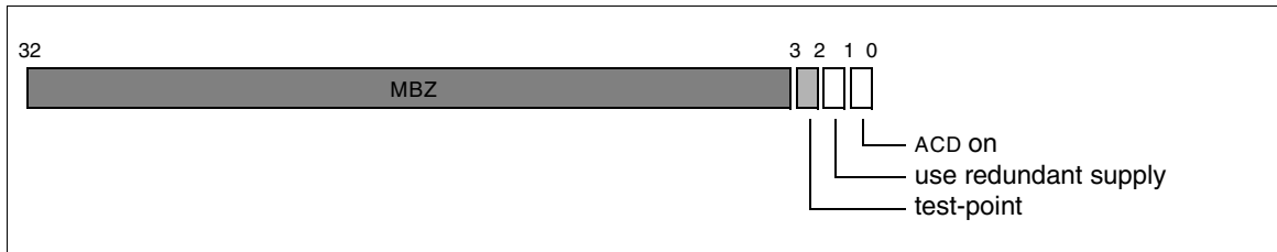
Figure 7 Power supply switching for the ACD
