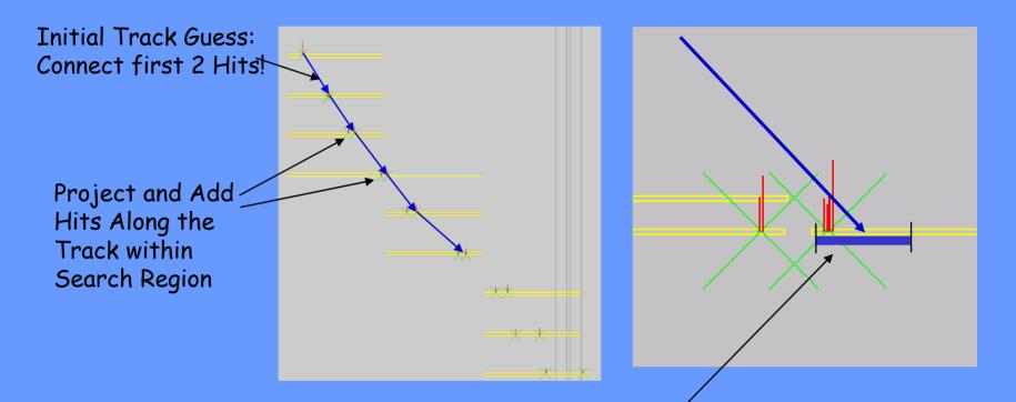
The search region is set by propagating the track errors through the GLAST geometry.
