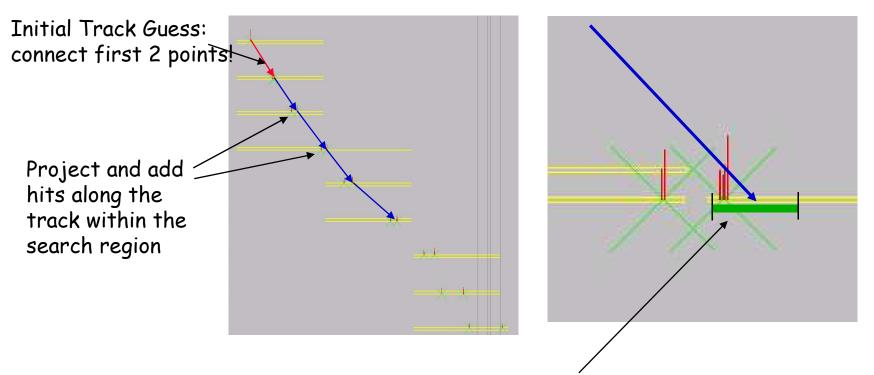
The search region is set by propagating the track errors through the GLAST geometry.
