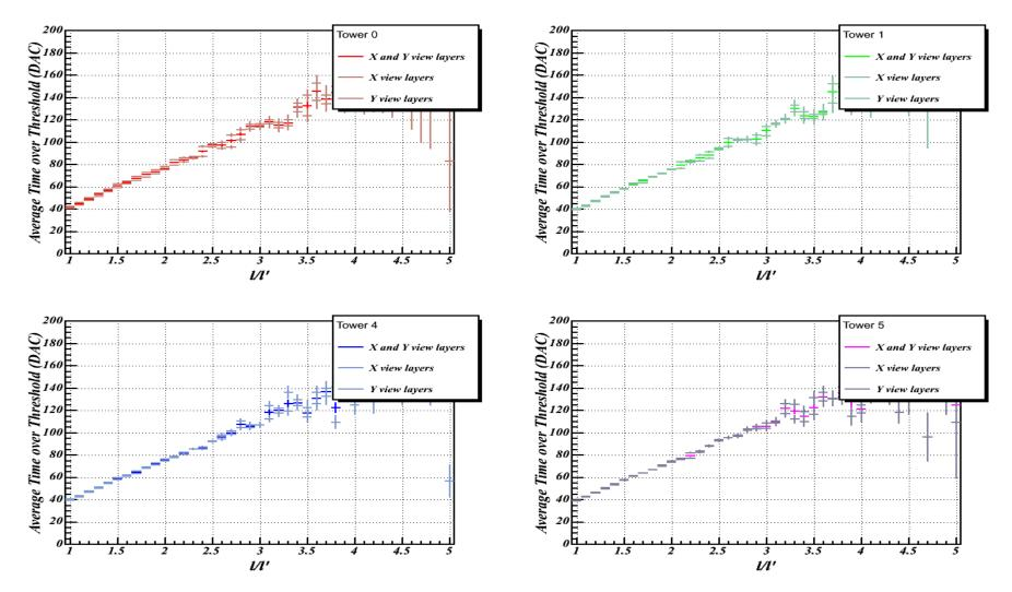
No significant differences in ToT vs l/l' between X and Y view layers
