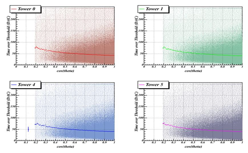
The ToT is minimum for vertical tracks and increases with  $\theta$
