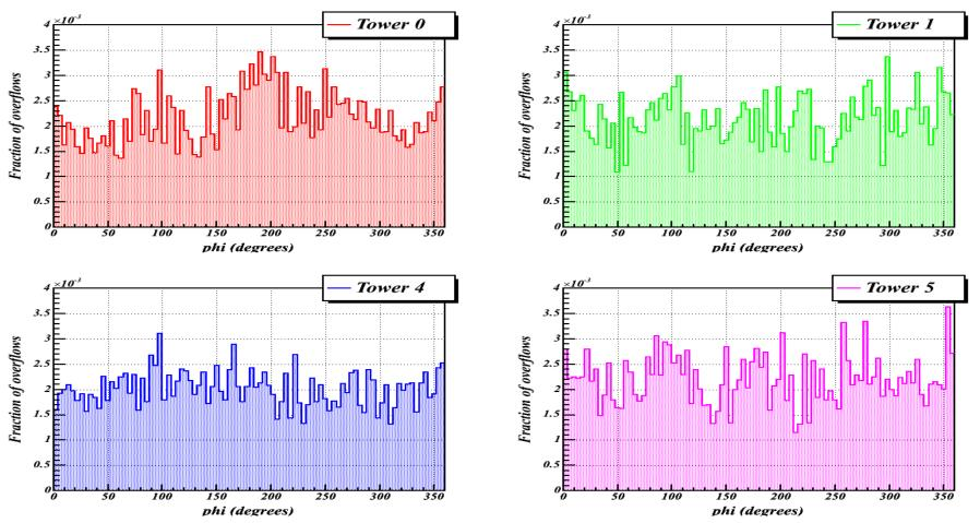
Fraction of overflows in Tower 0 seems to depend on  $\varphi$  with a period of 90°. This effect could be caused by small differences between the average behavior of SSDs in X-view and Y-view layers
