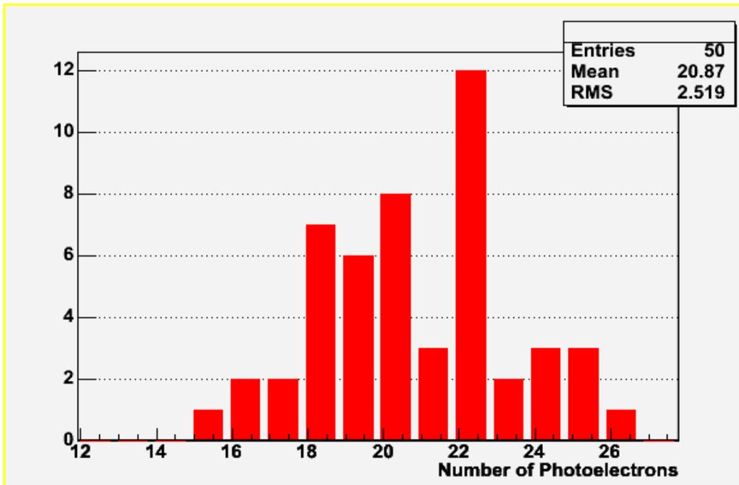
Alex used these results to determine indirectly the Light Yield of the side tiles of the ACD.
