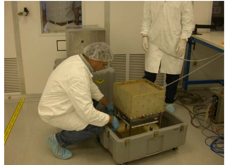
EM CAL ready to be hooked to the EGSE
