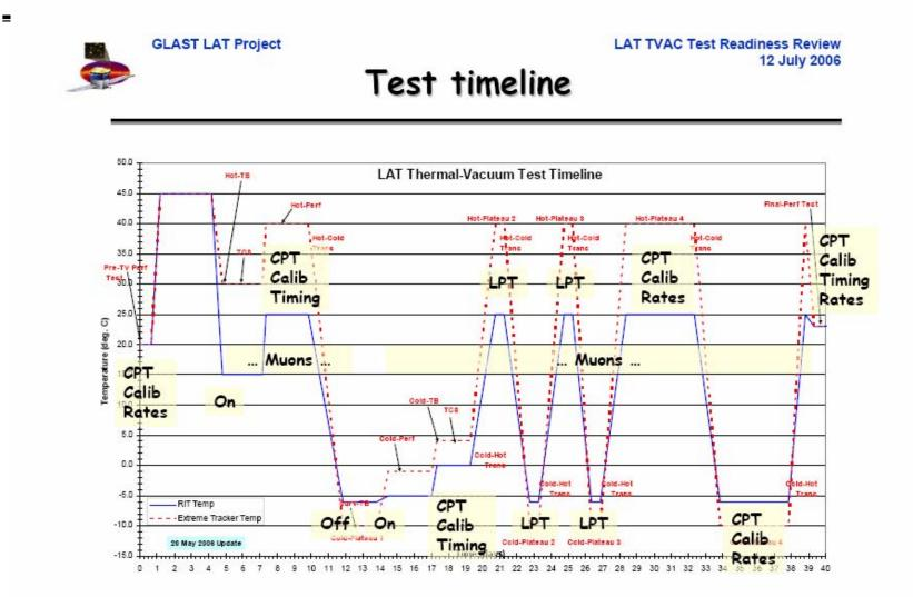
Instrument Functional Tests
