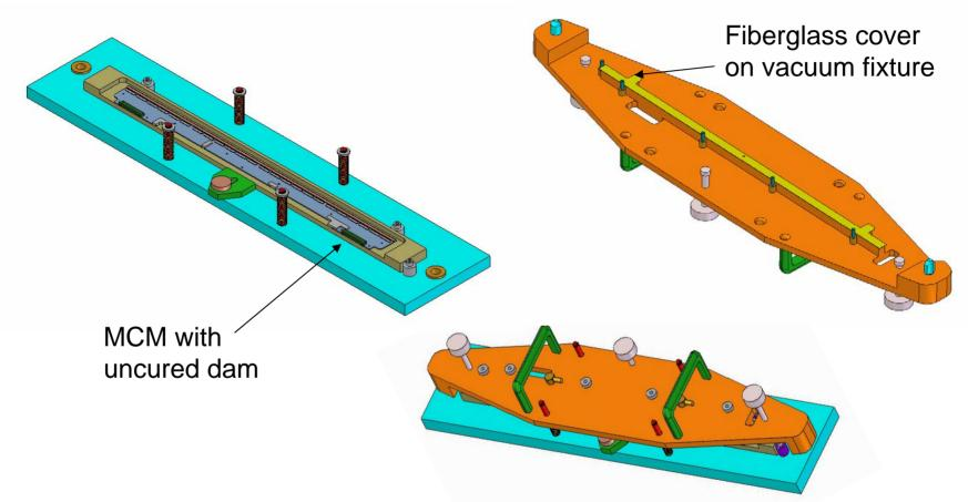
Design of a fixture for mounting a cover on top of the Hysol dam is in progress. This would be used in place of the encapsulation fill and would certainly eliminate the problem of encapsulation delamination breaking wire bonds.
