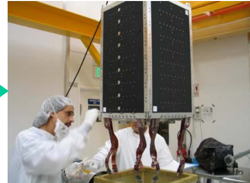
Installing into the single bay test stand
