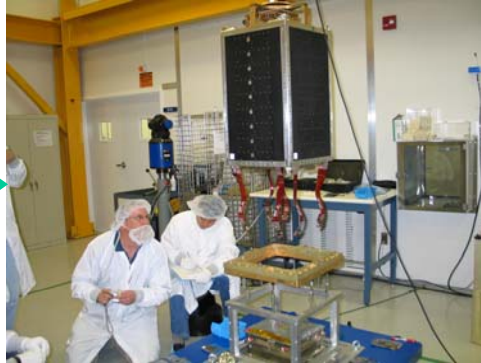
Lifting from the test support stand
