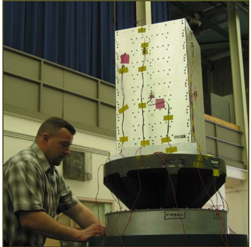
Prototype Tracker Vibration Test at NASA Ames
