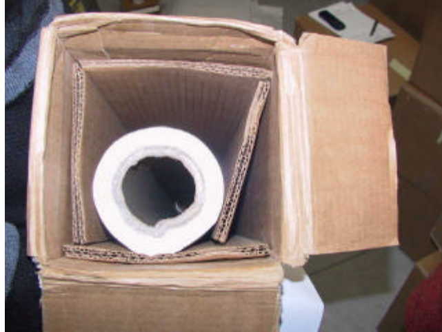
fig.2) The box was opened in Plyform first time. The Al roll inner cylinder is not regular, indicating shoks.
