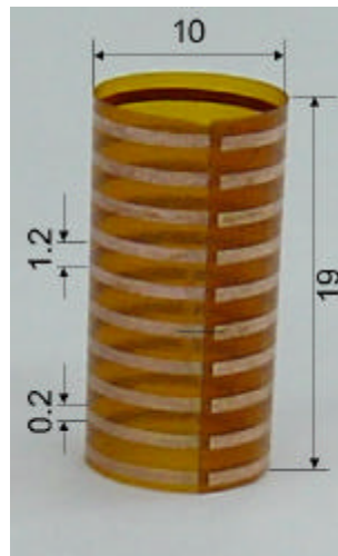
Fig.1 The Kapton cylinder. Units mm
