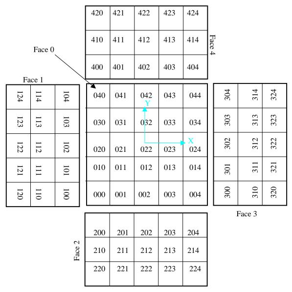
A fourth digit, the most-significant digit, gives the PMT channel (primary or redundant), or the layer number in the case of the two-layer design. In the two-layer design, the inner layer is layer 0 and the outer layer is layer 1. The figure therefore shows the numbering for the inner layer or the primary PMT. The complementary layer or PMT would have a "1" in front of every number in the figure.
