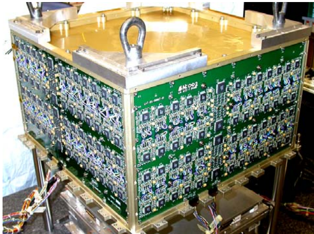
Figure 2: Calorimeter Engineering Model Assembly
