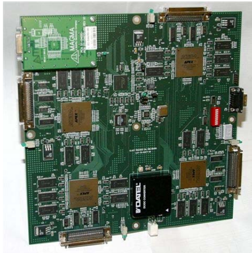
Figure 4: Front-End Simulator Board
