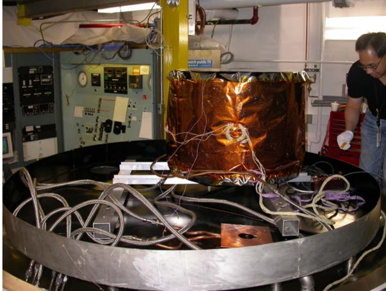
Figure 1: Calorimeter Engineering Model is enclosed in a thermal shroud and mounted on the thermal vacuum chamber base plate.
