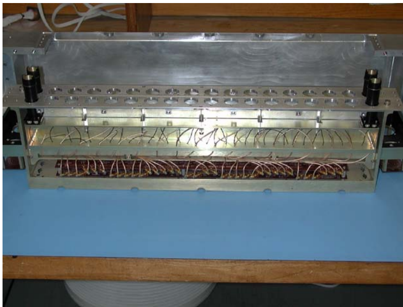
Figure 2: Engineering Model ACD electronics chassis being used for fit testing of the phototubes, high voltage bias supplies, and FREE cards.
