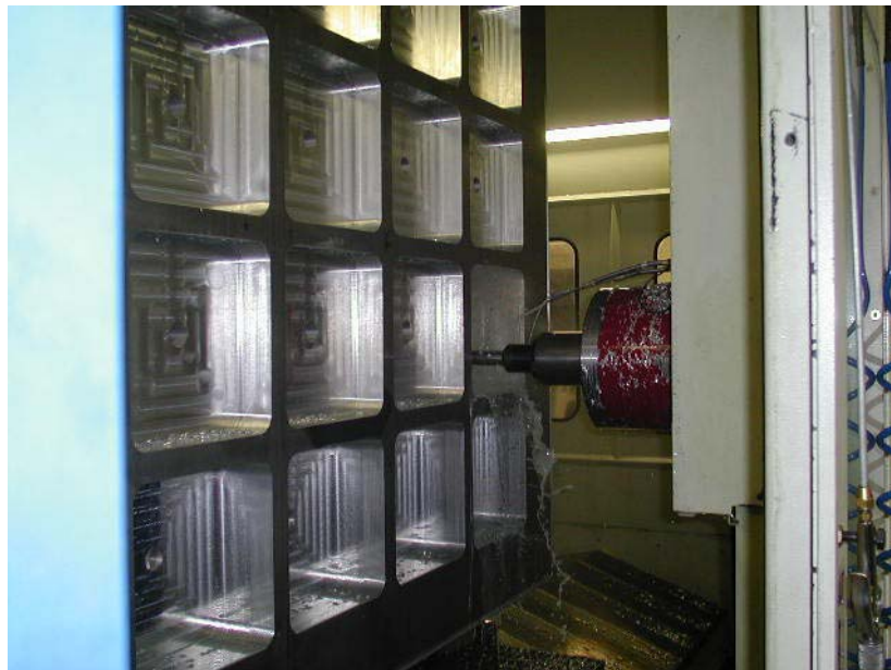
Figure 1: Grid being rough-machined.
