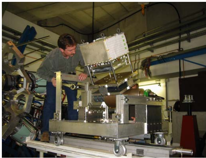
Figure 2: Calorimeter EM on translation and rotation test fixture at GSI in Darmstadt, Germany.
