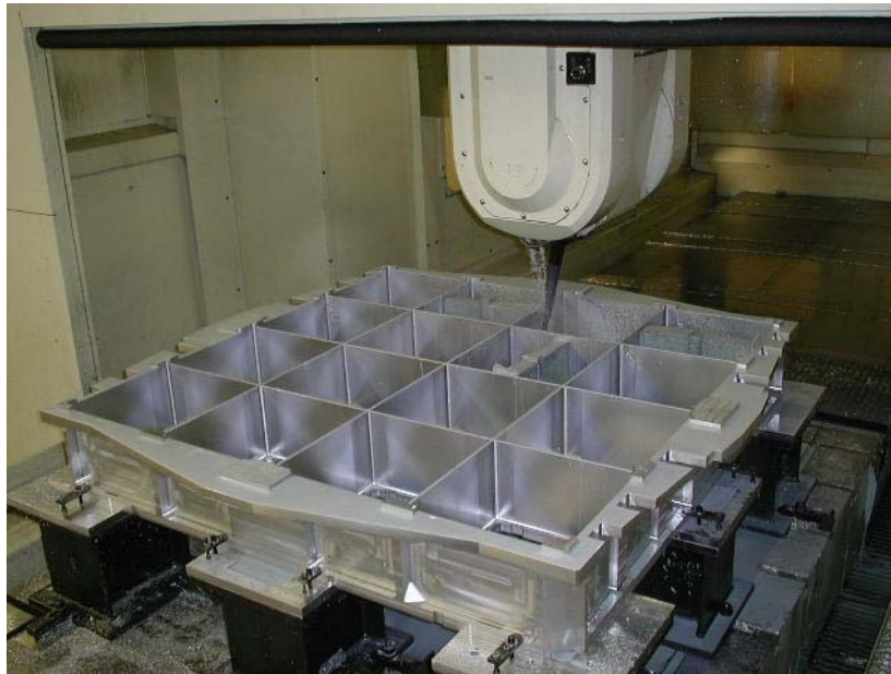
Figure 2: Machining of First Grid
