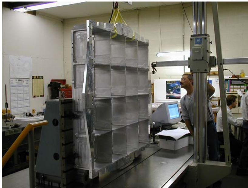
Figure 4: First grid on the coordinate measuring machine at Tapemation.
