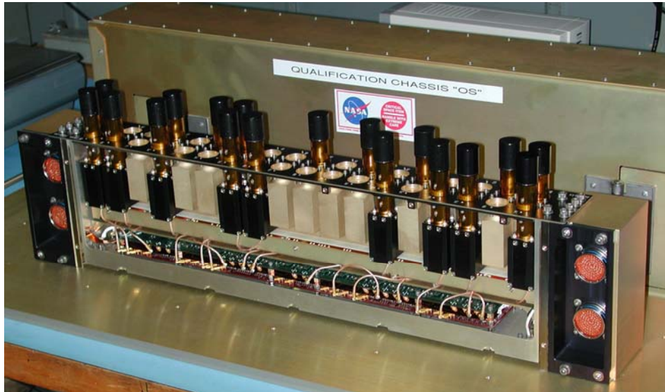
Figure 3: ACD qualification electronics chassis.
