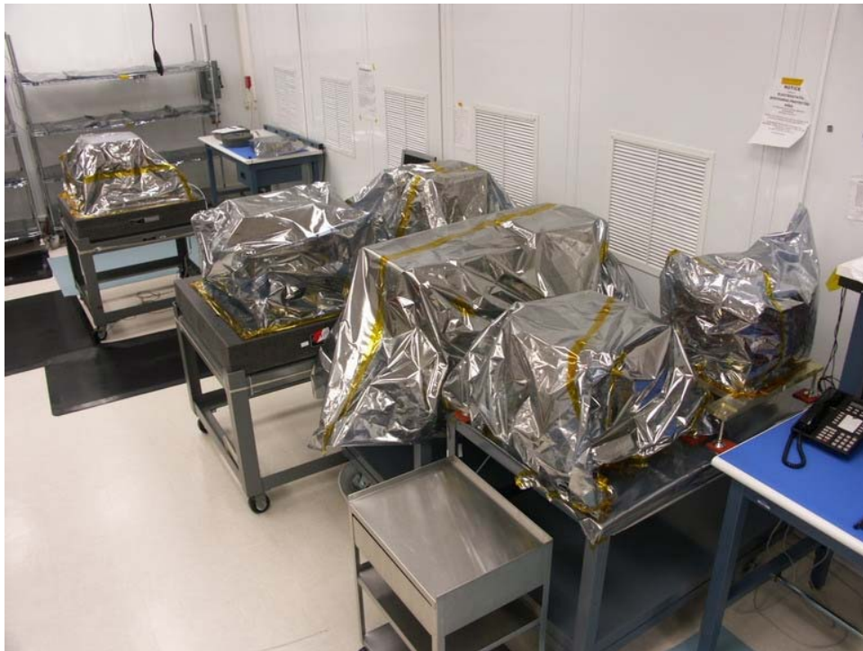
Figure 2: Seven completed CAL Pre-Electronics Modules are in storage awaiting installation of electronic cards. The completed PEMs have been tested using EGSE to verify the performance of the 96 CDEs in each using cosmic muon signals. Each PEM is stored under an ESD tent with dry nitrogen flow.
