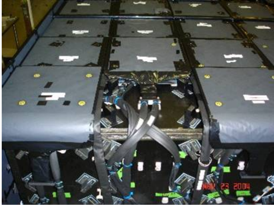
Figure 2: Clear fiber routing and ribbon detectors under a bent TDA, before the last top tile was installed.
