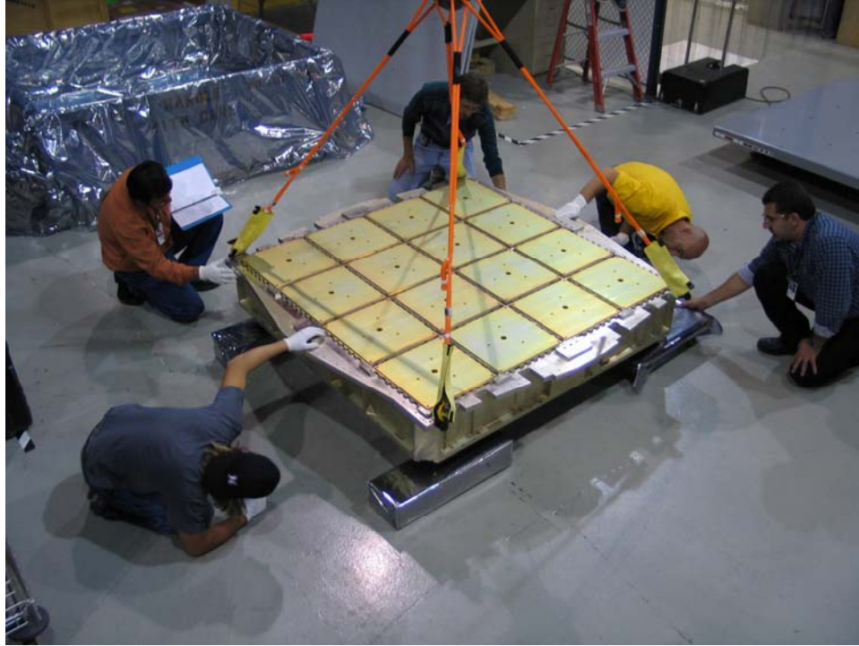
Figure 4: Moving the flight grid to the tilt-table.
