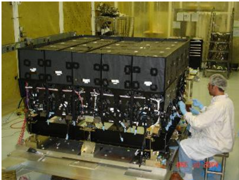
Figure 2: ACD with top and crown TDAs completed, working on second side row.
