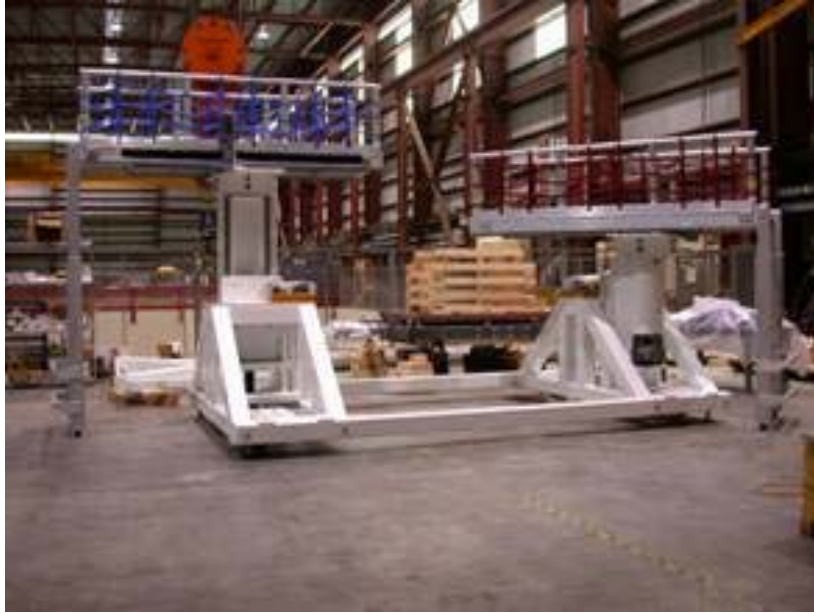
Figure 4: LAT integration stand with personnel access platforms installed.
