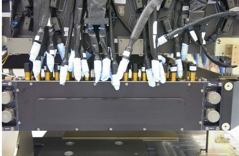
Figure 3: First electronics chassis installed on the ACD.
