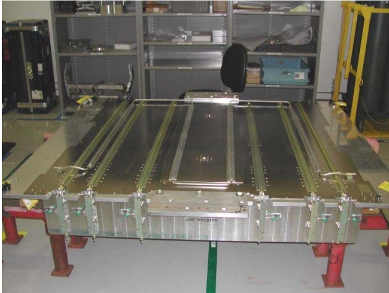
Figure 4: X-LAT plate fit check on bonding fixture.
