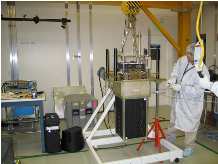
Figure 5: Inserting a flight Calorimeter into the 1x1 grid to complete the first flight tower for electronic testing.
