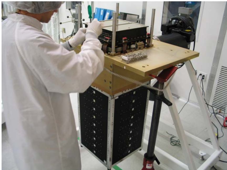
Figure 2: Second tower in the single-bay grid, being prepared for electrical testing
