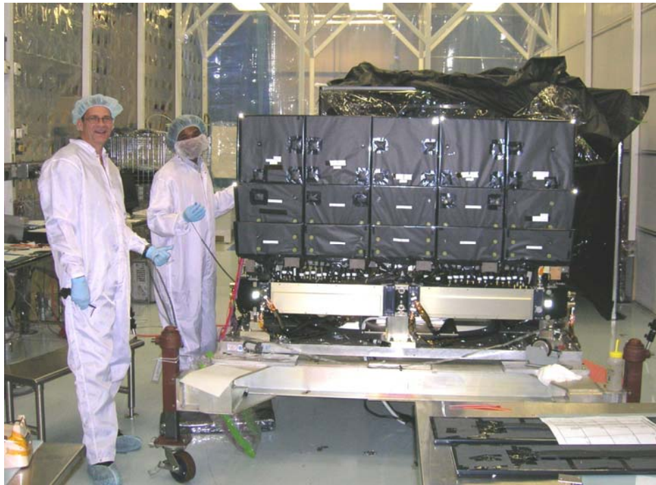
Figure 2: Three rows of ACD tile detectors assembled.
