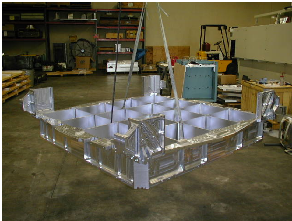
Figure 3: Second grid machining completed.
