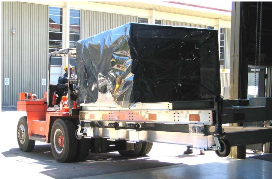
Figure 1: The ACD on its shipping dolly being brought into the LAT Integration and Test Facility.
