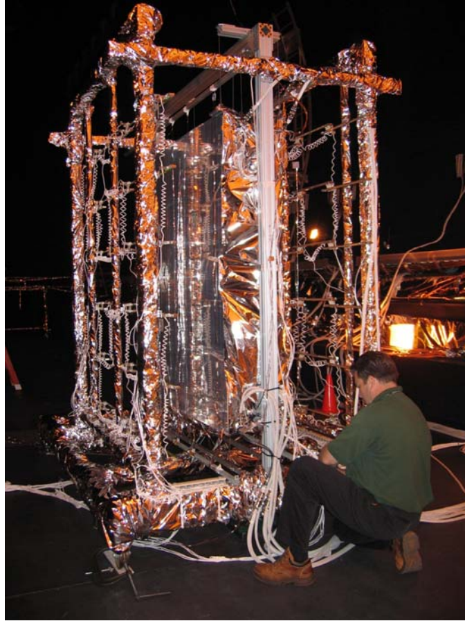
Figure 2: Radiator in thermal vacuum test preparations.
