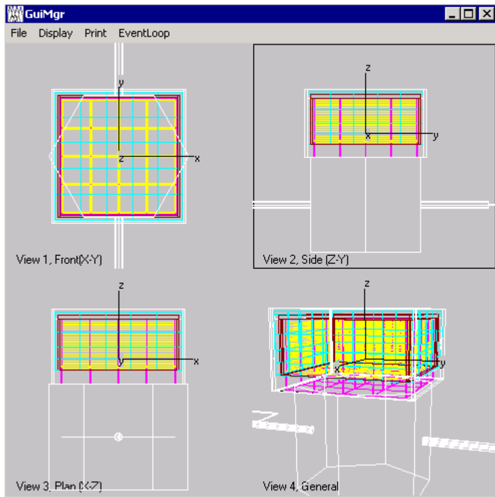
Figure 10.3.2.1. The full GUI display, with pull-down menus for control of the job, and four projections of the instrument, showing the outer shield (white outline), ACD tiles (blue rectangles), TKR system (yellow), CAL (below the TKR). The Spacecraft is represented by a hexagonal solid. The solar panels are shown as well.
