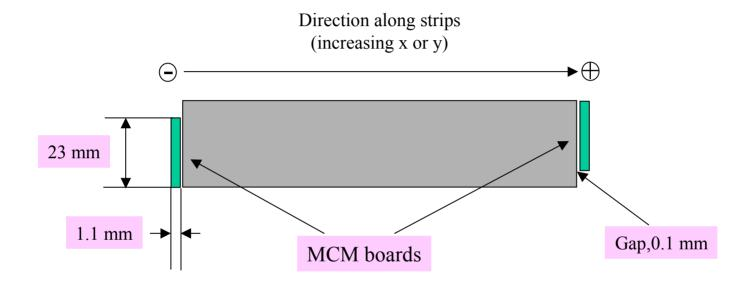
The MCM board a the positive x/y end of the tray feeds the top layer of Si Strips, and the one at the negative end feeds the bottom layer.
