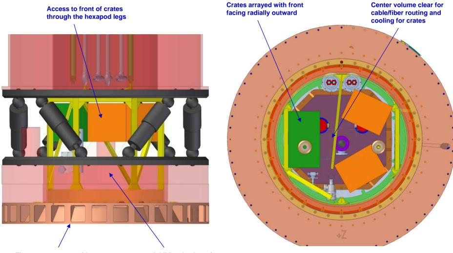
The camera rotates with respect to the hexapod, so if needed we can rotate the camera to align a crate with an opening in the hexapod Additional volume is available, but the access is much more limited
