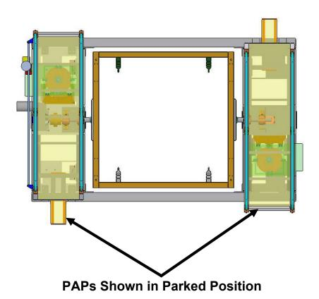
Limit Switches prevent power from being supplied to PAP Drives Unless LAT is Level within ± 1° (TBC)
