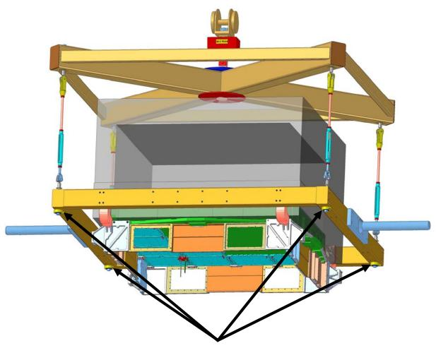
0 to 10K lb "Donut" Load Cells, Under GPR, 4 Places, to Allow Adjustment of Turn-Buckles for Balanced Lift (TBR)
