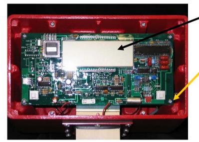
Remove Circuit Card; 4 Screws, 1 at each Corner
