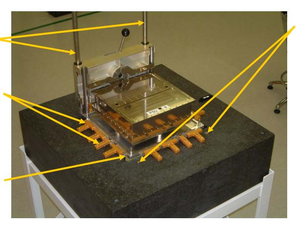
Extra Set of Alignment Rod Receptacles in Case 1<sup>st</sup> Set Gets Damaged
