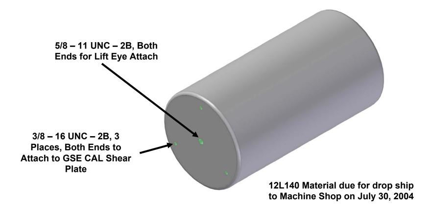
\*Note: Nickel Plating is much lower cost than Powder Coat
