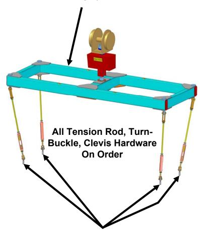
1/2 - 20 UNF – 2A Spherical Tie Rods In House
