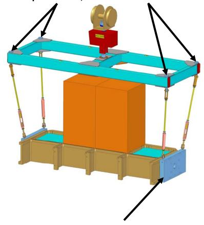
1x4 Grid to Support Shaft – Flange Interface Plates are Ready for Match Location
