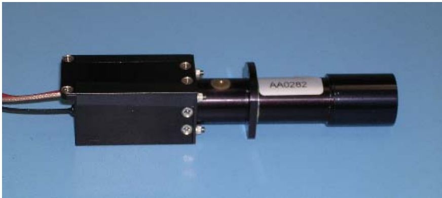
Completed PMT Assembly – Functionally and light tight tested AntiCoincidence Detector (194 required)
