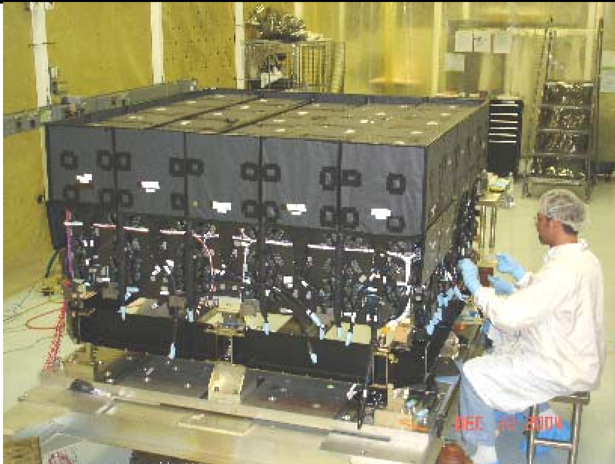
Top and Crown TDAs completed, working on 2 nd side row
