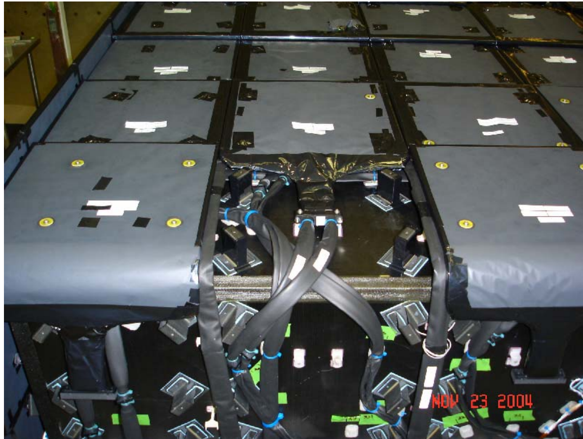
PICTURE SHOWING CLEAR FIBER ROUTING AND RIBBON DETECTORS UNDER A BENT TDA
