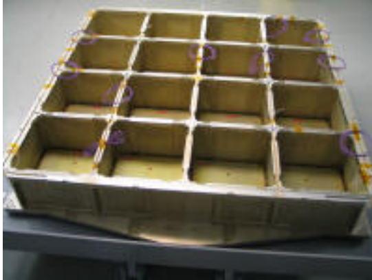
Grid thermocouple bonding and purge tube installation complete.
