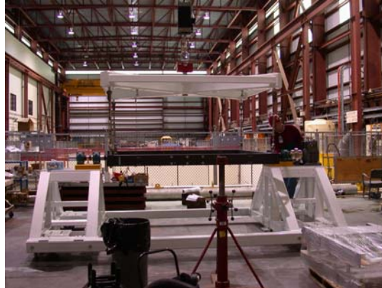
4X4 Z-axis Vertical Lift Fixture Proof Test Complete
