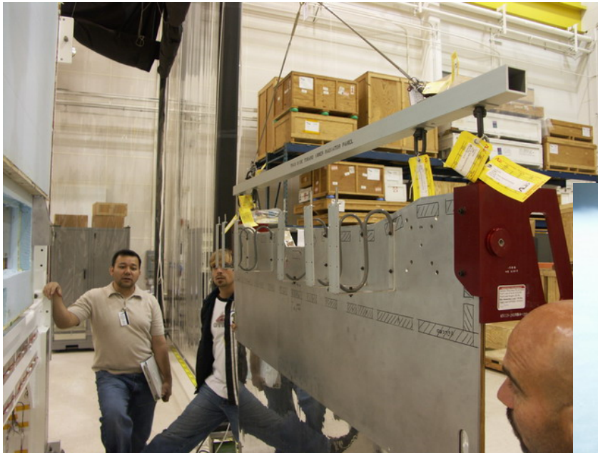
Radiator installation test
