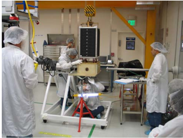
Removal of TKR A from the Single Bay Stand
