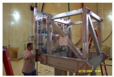
Both radiators delivered to Acoustic Test Facility
