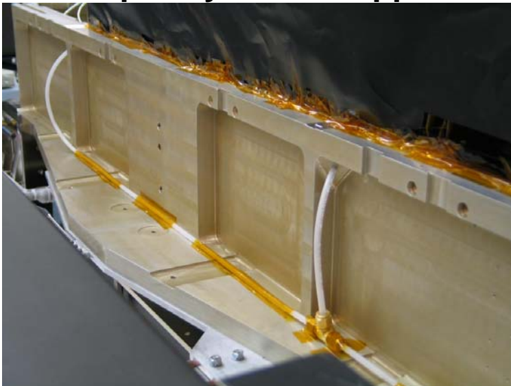
Purge Tube Installed
