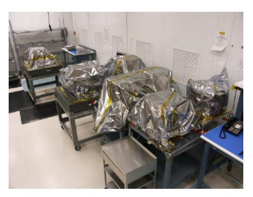
Seven completed PEMs in ESD covers await electronics for completion of CAL modules.
