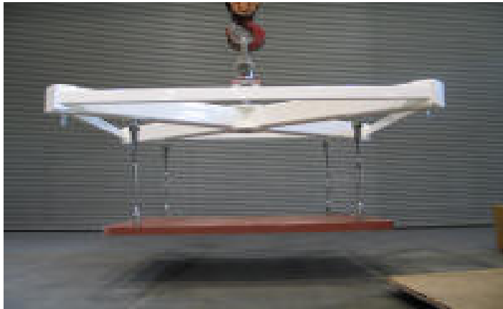
4x4 Lift Fixture with a proof test weight
