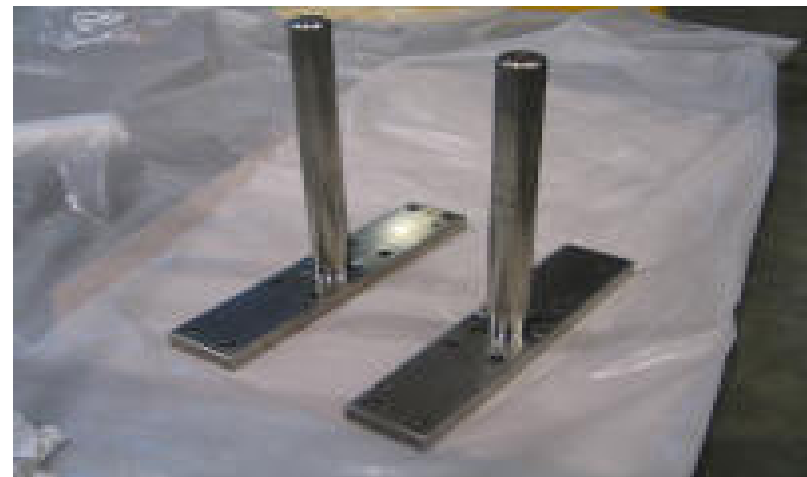
Grid Perimeter Ring Support Shafts
