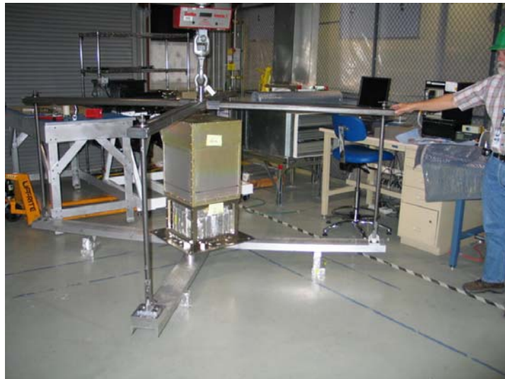
ACD lift fixture proof test 4.1.9 - Integration and Test
