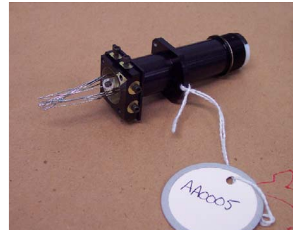
PMT Bonded in mechanical housing
