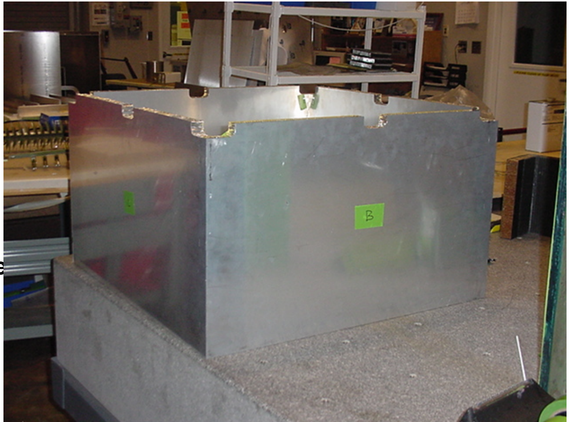
1/2 SCALE ACD SHELL ASSEMBLY – BEING ASSEMBLED TOP SIDE DOWN
