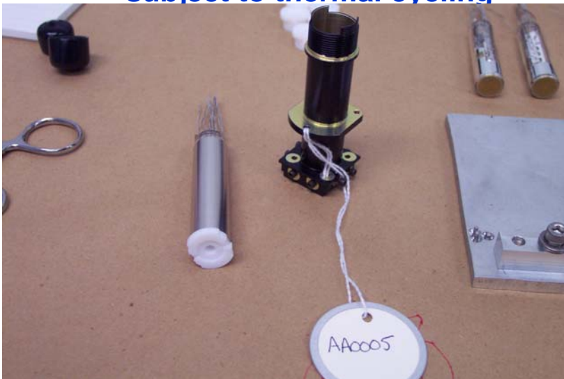
Preparing for PMT bonding
